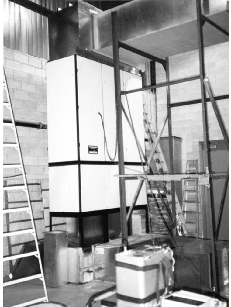
Mock-up of prototype air-conditioning unit for testing.
