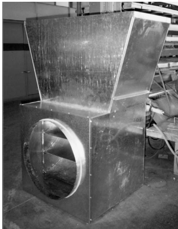
Axial return fan silencer component: Rectangular-to-round transitional elbow silencer with turning vanes.
