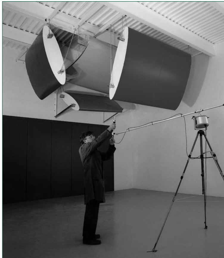
Vibro-Acoustics' 20,000 cu.ft. reverberation chamber, double the industry norm, is designed for more accurate low frequency measurement.
