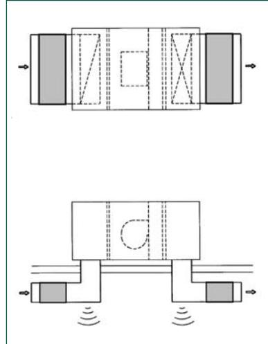
Roof Top Unit with standard silencer has breakout noise problem.
