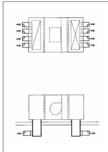
Round duct solution to breakout problem is costly because of the manifolds required and the multiple duct runs.
