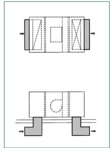
Elbow Silencers with HTL casings reduce breakout noise and also provide downstream attenuation.
