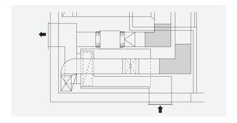
Above: Simplified plan drawing (adapted from original) Left: Mechanical equipment room. Plan view. Right: Elbow silencers installed in equipment room walls to reduce breakout noise.
