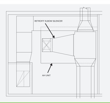
Mechanical room drawing (plan view) shows existing ductwork and complex fitting replaced by the elbow transitional silencer.
