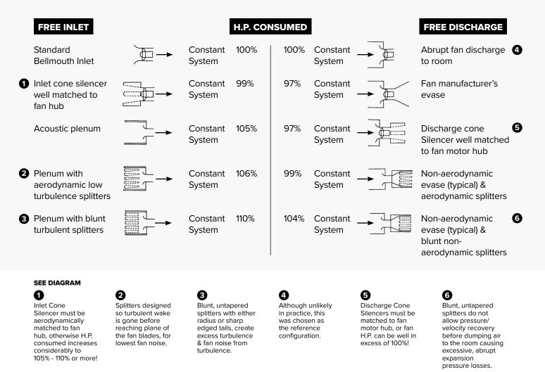
**General Notes: A.** If a fan consumes less horsepower, it generates less noise and therefore needs less silencing. **B.** Turbulence allowed to impinge upon the plane of the axial fan blades can create 10-15 dB or more excess fan sound power.
