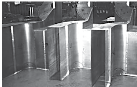
Left: Internal perforated metal air passages for T discharge silencers are shown before installation into silencer casings and glass fiber packing. Right: AHU discharge silencer on its side. One duct connection is on the left and AHU connection is on the right.
