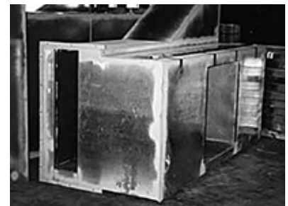
Left: Internal perforated metal air passages for T discharge silencers are shown before installation into silencer casings and glass fiber packing. Right: AHU discharge silencer on its side. One duct connection is on the left and AHU connection is on the right.
